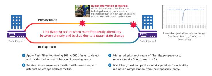
This innovative, VIAVI patented feature is uniquely designed to assist in troubleshooting network flapping. It provides a time stamp of the attenuation event to be correlated to route flapping or error events in your NMS or router topology table. Customers are able to see the location of these events and advance the troubleshooting process dramatically by detecting and locating ISDFs caused by flash attenuation events, which is especially critical for high-speed rates.
